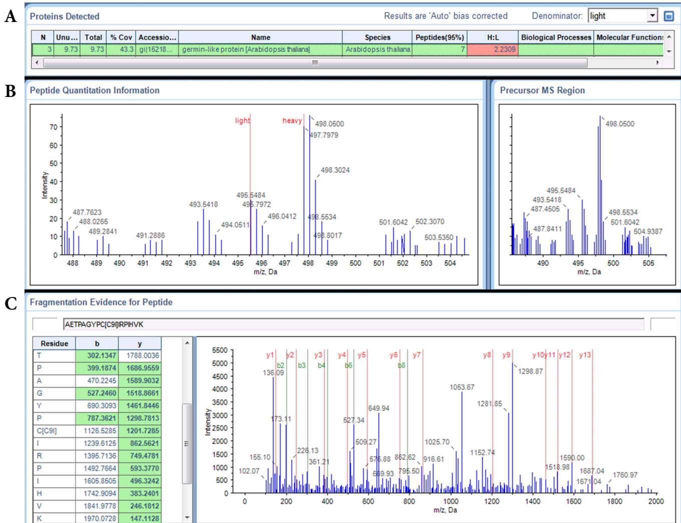
Figure 3. Example of protein identification and quantification result including summary of the protein (A), peptide quantification in the control sample (light) and ABA treated sample (heavy) (B), and peptide MS/MS spectrum indicating heavy ICAT labeled cysteine (C).
